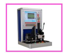
Testing for small die-cast rotors managed by PC. Maximum dimensions: Ø 120 mm, H 150 mm with and without shaft. Manual loading and unloading. Cycle time 10".
